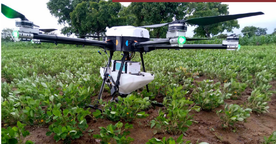
Drone-supported application of Aflasafe to groundnuts in Burkina Faso
